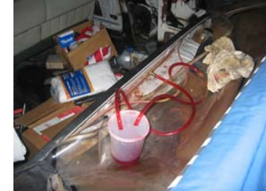
a "transfusion" of fresh hydraulic fluid to the pump cylinders
